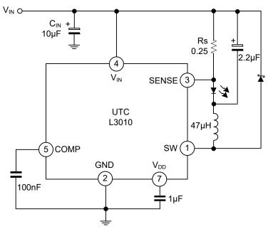
$6 \sim 40V$  input voltage, 350mA output LED driver
